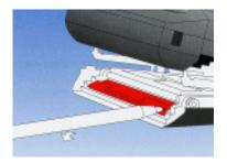
the film pack first. Insert the tip of a ballpoint pen into the small square in the red bar as shown. Pivot the red bar out of the way for access to both rollers. Clean the rollers with a lint-free cloth or a cotton swab dampened with water while manually turning the roller gear with your finger.
